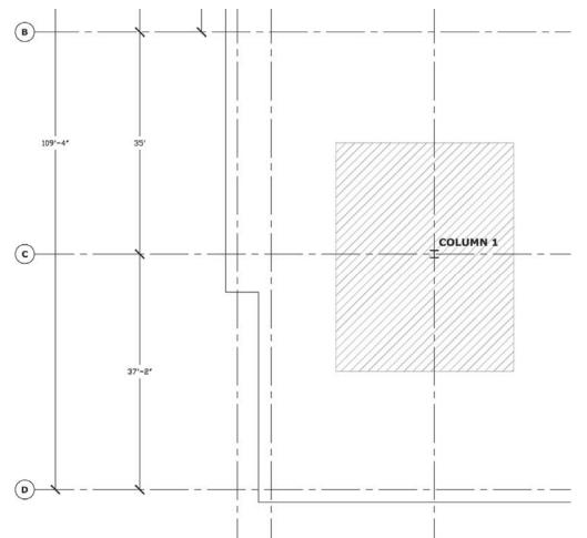
The tributary area method was also used in determining the loading on "column 1"; Live load reductions were not considered in the design of the column. Second order effects were also not considered in the design of the column. The hand calculation of "Column 1" can be found in the appendix and is labeled hand calc. - 1.
