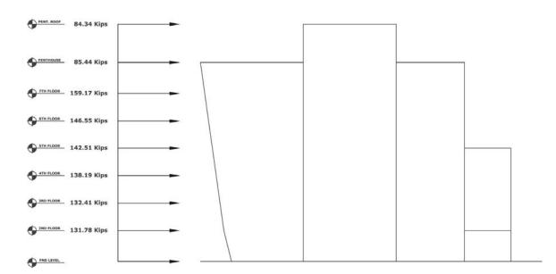
The preceding image shows the distribution of the factored wind shear on each level. The factored wind shear is equal to 1.6 \* the wind shear, this was then compared to the factored seismic shear which has a factor of 1 in the load cases discussed in this report.
