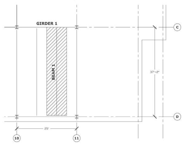
For this case I determined that the live load was reducible and ended up with a design live load of 85.27 PSF which is within the allowable limits of 0.5 \* the original live load.
